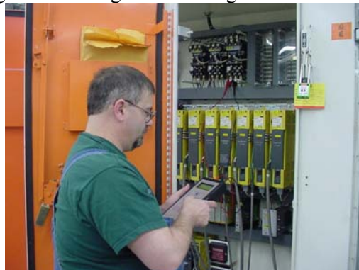
Figure 7: Testing A Machining Center with MCA
