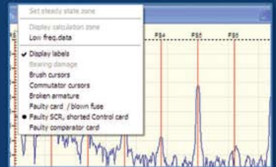
ATPOL II Automatically Identifies and reports Common DC Motor faults, such as broken armature, faulty SCR's, etc.
