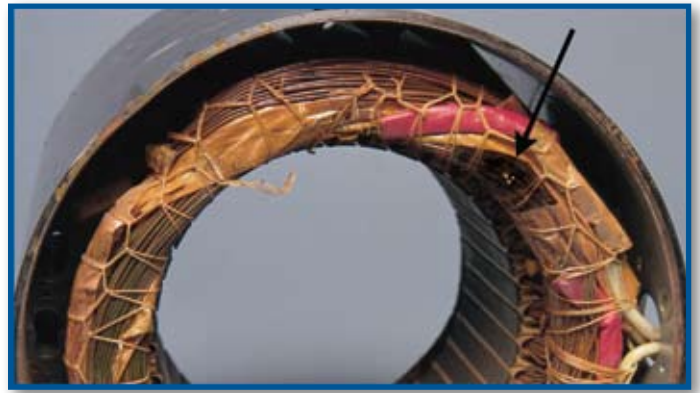
This winding fault was caused by a voltage surge. An insulation test will not detect it!
